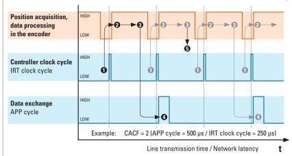
Clock specification by controller IRT clock cycle = Transmit clock
