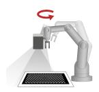
The "Hand-Eye calibration (Robotics)" calibration method is used to determine the reference between Tool Coordinate System (TCP) and Camera coordinate system (position and orientation) when the VISOR® is attached to the gripper.
