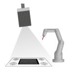
The calibration method "Calibration plate (Robotics)" is used to determine absolute positions in the robot coordinate system. This is done by acquiring one or more images of the calibration plate and teaching four fiducials.
